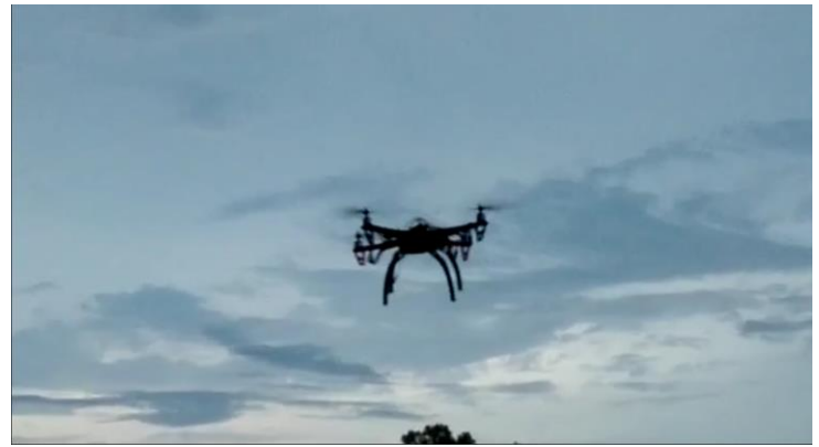
Fig 5.5 Test flight of custom built APM based drone with autonomous navigation
