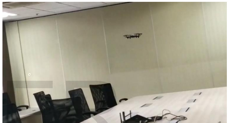
Fig 5.6 Test flight of parrot mini drone with control system implemented in Simulink
